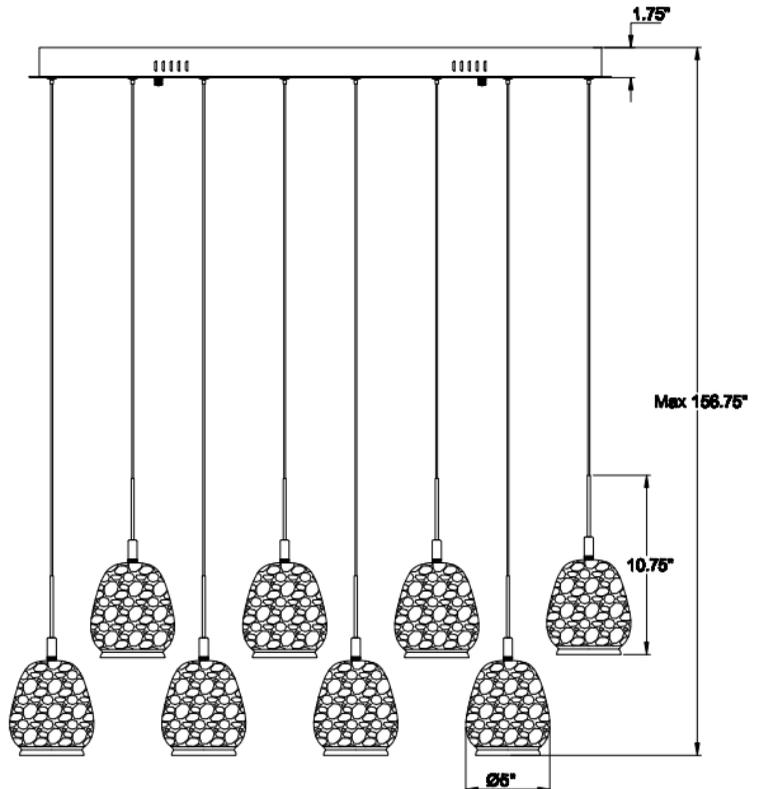
Fixtures weighing 35 lbs. or more must be supported and installed independently of the ceiling outlet (junction) box and require additional support in the ceiling where the fixture is being installed
